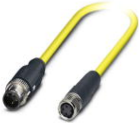
Sensor/Actuator cable, 3-position, PVC, yellow, shielded, Plug straight M12-SPEEDCON, A-coded, on Socket straight M8, Cable length: 1.5 m
